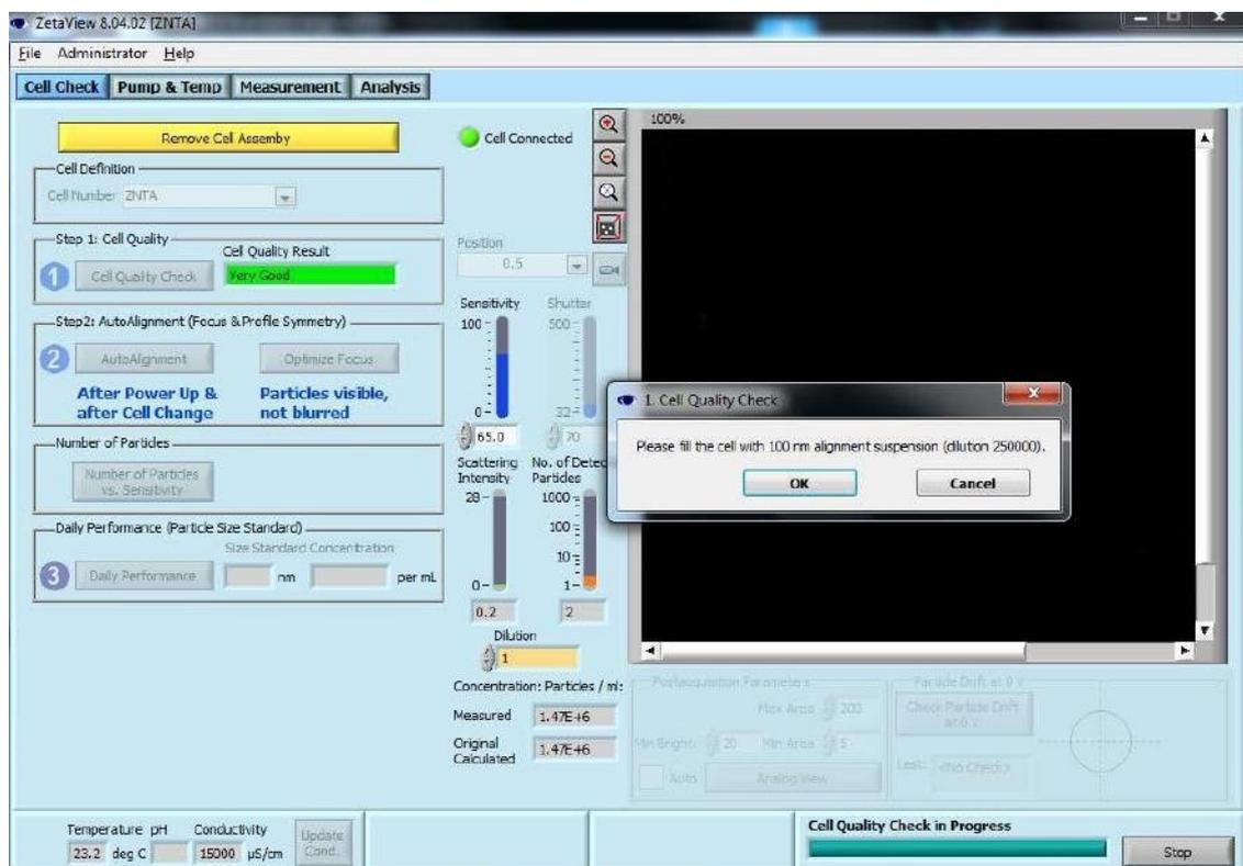
10. CellCheck 合格后，会出现“Please fill the cell with 100nm alignment suspension (dilution 1: 250,000)”的消息提示。
